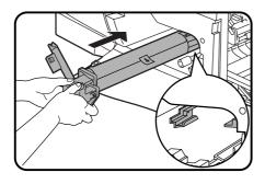
Remove the new drum cartridge from the protective bag and gently insert the lead end of the drum cartridge along the guides.
