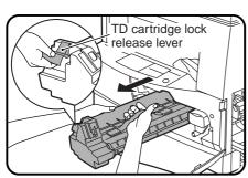
3 Lift the TD cartridge lock release lever and pull the cartridge out until the green strap handle can be grasped by the right hand. Lift the cartridge by the handle while supporting it with the left hand at the green label position to remove it.
