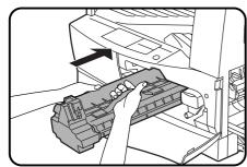
Close the front cover by pushing both sides with your hands and then close the side cover by pressing the handle on the cover. The : indicator will go out .
