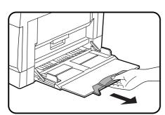
When feeding 8-1/2" x 14" or 11" x 17" sized paper, extend the bypass tray.
