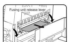
Carefully remove the misfed paper. Lower the fusing unit release levers to allow easier removal. Return the release levers to their operating positions.
