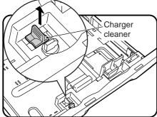
Gently lift and pull out the paper tray and take the charger cleaner out by holding the tab.
