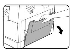
Unfold the bypass tray.
