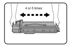
Remove the new TD cartridge from the bag. Hold the cartridge on both sides and shake it horizontally four or five times.
