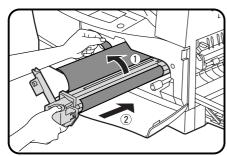
Remove the protective cover from the drum cartridge and then push the cartridge all the way into the copier.
