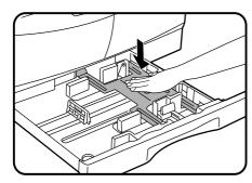
**7** Push the pressure plate down until it locks in place.
