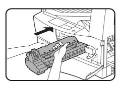
Gently install the TD cartridge. To install the TD cartridge, see page 24, TD CARTRIDGE REPLACEMENT.
