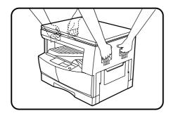
Be sure to lift by the handles on both sides of the copier by two persons to unpack the copier and carry it to the installation location.
