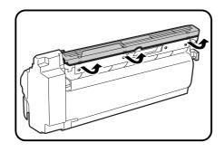
Remove the protective cover from the TD cartridge by unlatching three cover hooks from the holes on the cartridge and then pulling the cover in the direction indicated by the arrow in the illustration.
