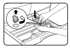
Remove the pressure plate lock. Rotate the pressure plate lock in the direction of the arrow to remove it while pressing down the pressure plate of the paper tray.
