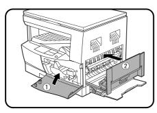
Close the front cover by pushing both sides with your hands and then close the side cover by pressing the handle on the cover. The drum replacement required ( ) indicator will go out.
