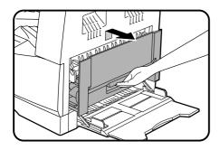
Open the bypass tray. Lift slightly on the side cover and slide the cover out until it stops.
